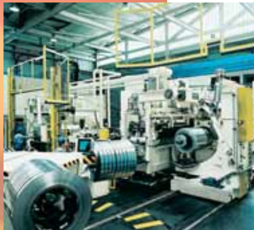
Top: One of the showpieces of the Werdohl works: the new 20-roll foil rolling stand.
