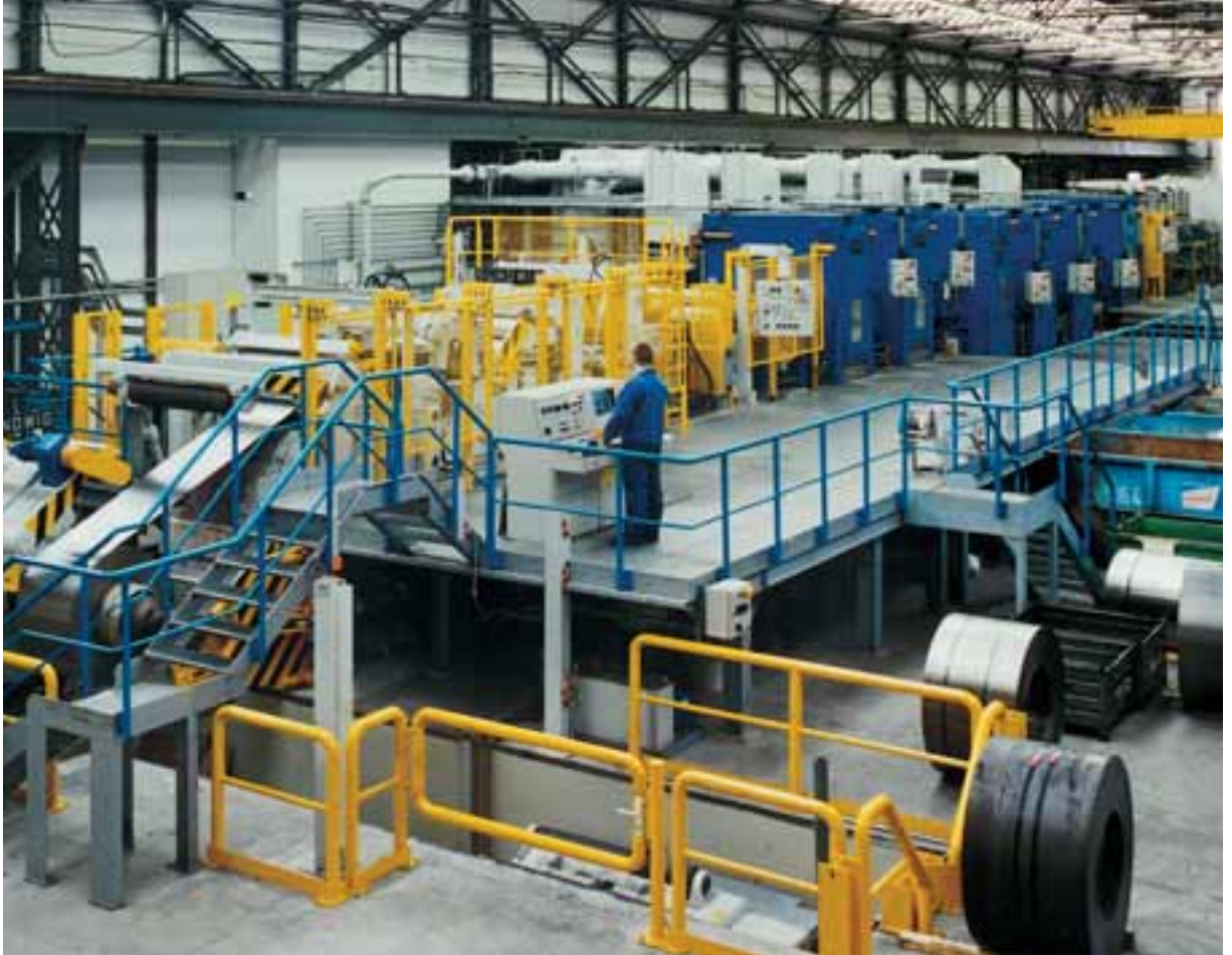
Precision grinding unit for processing pickled and roughed hot strip material; this is the last preliminary stage for the downstream cold rolling process.
