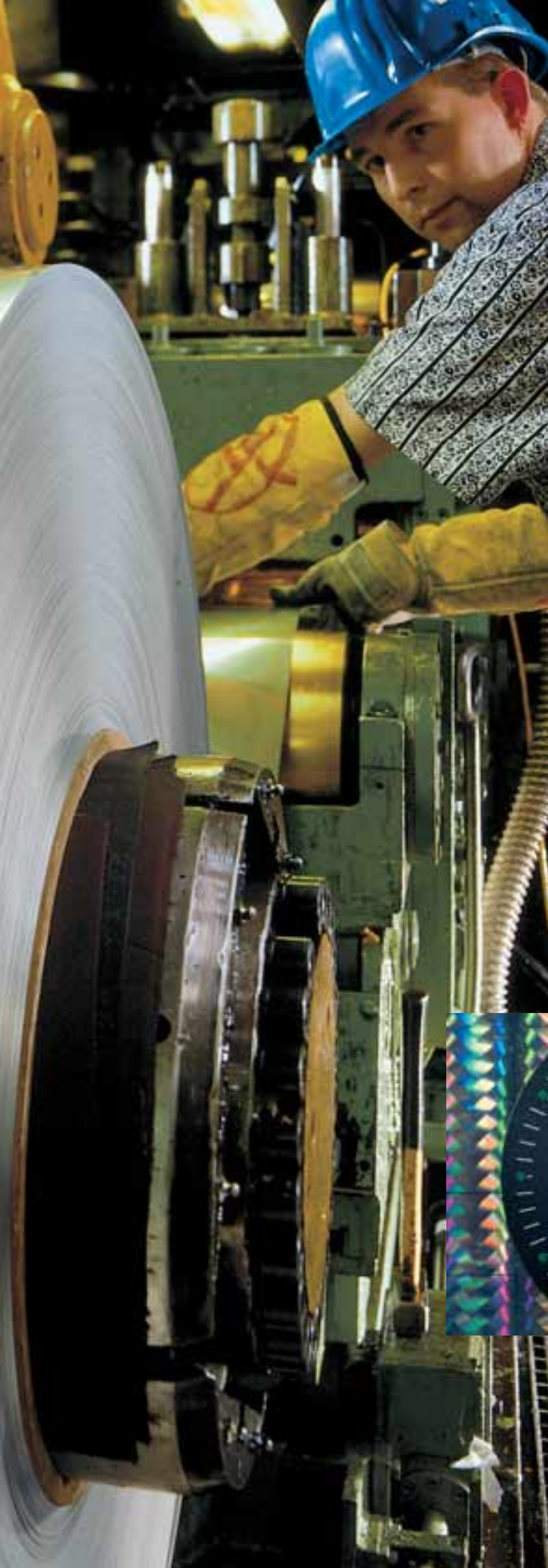
Left: The 6-roll precision reversing mill is capable of producing narrow strip with extremely tight dimensional tolerances.
