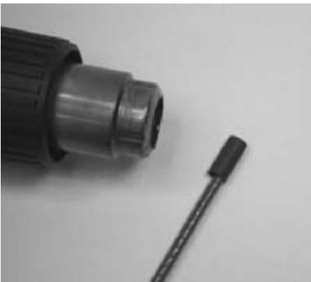
2. Crimp tube 6/2, L = 20 mm is pulled in over the end of the cable to the edge of the removed outer sheath. 5 mm of the crimp tube must still be free of the cable.
