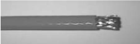
1. Remove 15 mm of the outer sheath.
