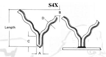
Nelson S4X studs are available in lengths up to 8.000" before weld length. After weld length is approximately 1/8" less than the before weld length.
