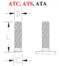
Mild steel studs are copper flash plated, stainless studs are passivated, and aluminum studs are acid etched for superior weld results.
