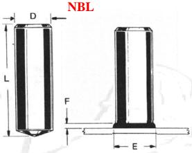
Special secondary operations, such as cross-drilling, grooving, heat treating, and pointing, can expand the application possibilities of Nelson NBL studs.
