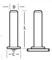
For superior welding results, mild steel studs are copper flash plated, stainless studs are passivated, and aluminum studs are acid etched.
