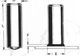
Special secondary operations, such as cross-drilling, grooving, heat treating, and pointing, can expand the application possibilities of Nelson NBL studs.
