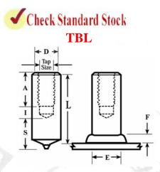
Reduced base studs are available but depth of tap drill point should not pass below shoulder of reduced diameter shoulder so that stud strength is not compromised.
