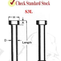
Shear connectors are typically used in composite steel construction for holding concrete slabs to steel members to resist shear forces and increase shear loading capacity in steel buildings, bridges, columns caissons, containment liners, etc. They also act as embedment anchors on miscellaneous embedded plates, frames, angles, strip plates, attachments and connections. Options for Welding Through Metal Deck are available for this stud.
