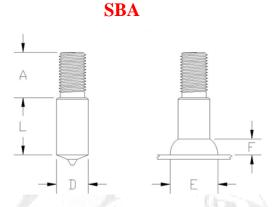
Nelson SBA studs are welded using ceramic ferrules in conjunction with argon as a shielding gas. The shielding gas is introduced through a gas foot assembly, #751020000, which is used for all diameters of SBA studs. Gas hose #515001001 and a gas regulator #514001001 are needed to deliver and control the gas flow from a pressurized cylinder.
