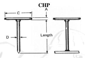
The pins may also be welded to cellular sheet metal deck to guarantee permanent anchorage of the sprayed fireproofing which protects electrical wires running through the cells, and provides added fire resistance per UL 263 and ASTM E119 standards, Fire Tests of Building Construction and Materials. In addition to securing the fireproofing, the pins also act as a reference gauge for the thickness of fireproofing to be applied.
