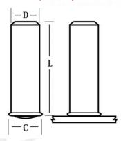
Unthreaded Stored Arc® studs are commonly used as locator or stop points. They may also be tapped with internal threads, or have smaller diameter externally threaded extensions
