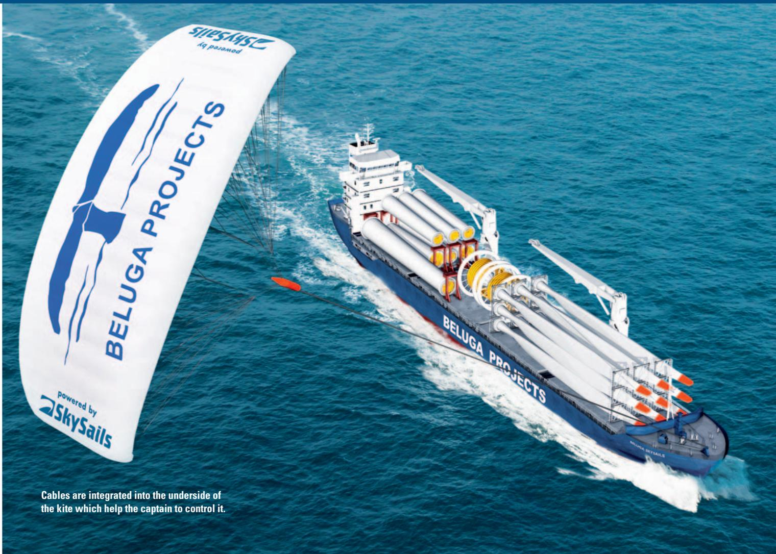
Cables are integrated into the underside of the kite which help the captain to control it.
