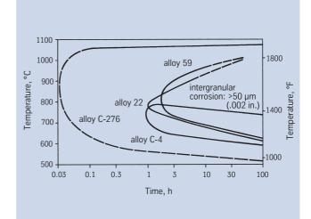
Fig. 2 – Time-temperature-sensitization (TTS) diagrams of nickelchromium-molybdenum alloys tested according to ASTM G-28 A.
