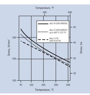
Fig.  $1 - R_{p0.2}$  yield strength for Nicrofer 5621 hMoW in comparison with other similar alloys.
