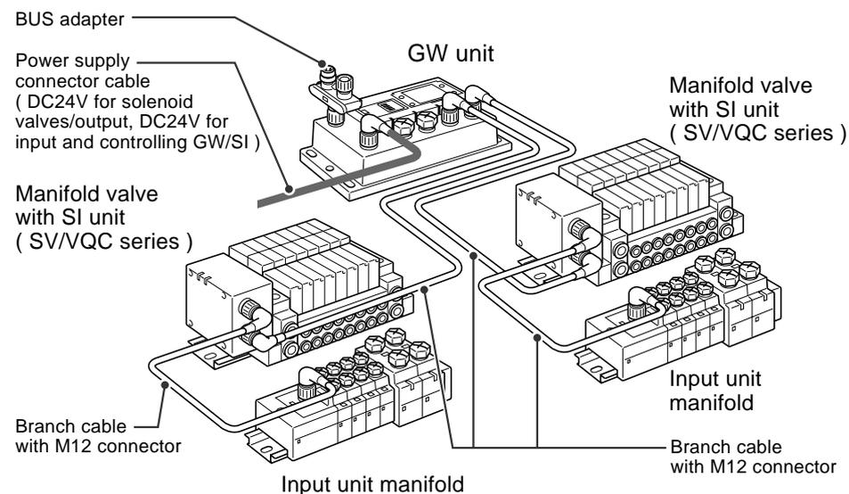
The reduced wiring system is connected to various kinds of fieldbus realizes the reduced wiring and decentralized installation of I/O devices . The signals to/from fieldbus are exchanged by GW unit, and the signals to/from decentralized I/O devices are collected and delivered by GW unit.
