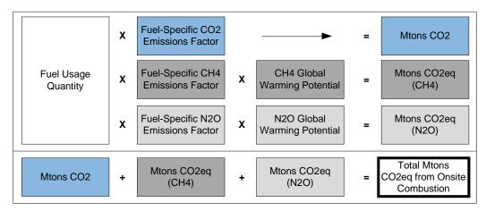
Figure 1: On-site Fuel Combustion Emissions Calculation
