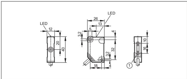
1: threaded insert M3, depth 5.8 mm, max. tightening torque 1.2 Nm (screw fixing class 8.8) when brass insert in contact with counterpart.
