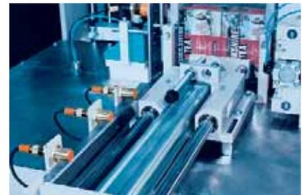
The sensor switches as soon as the magnet has reached the switch-on point. The direction of movement is not important.
