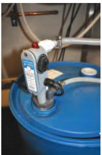
Pick-up tube with low level indicator
