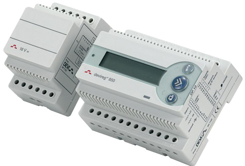
The devireg™ 850 is the most optimal solution for keeping an area free of ice and snow. devireg™ 850 acts on information received from the sensor(s) which register both temperature and moisture. devireg™ 850 calculates the information and secures that the heat only will be turned on when the right combination of low temperature and a certain level of moisture are detected. This gives an energy saving system and reduces running costs.
