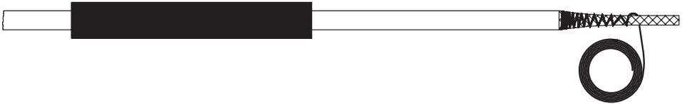
13. Pull the large crimp tube B over the copper protection screen and squeeze the end tight. Apply heat starting at the end so that the air is forced out of the crimp tube. Make sure that the glue is running out from the end of the crimp tube before stopping.
