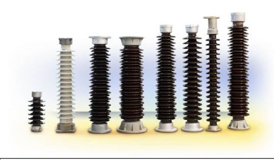
Post insulators for apparatuses and plants in conformance to IEC 273 to the voltage level of 420 kV. In this group of insulators, there is a wide range of products concerning voltage levels, strength and creepage distances. Construction is performed in conformance to IEC -273 and IEC - 815 or according to the customer's request. Voltage level range is 12-420 kV.
