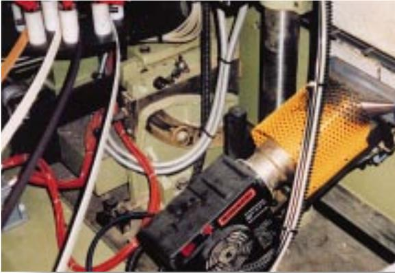
Hotwind S installed in a edge banding machine. These machines, from manual to large computer controlled models, require hot air to activate the hot melt.
