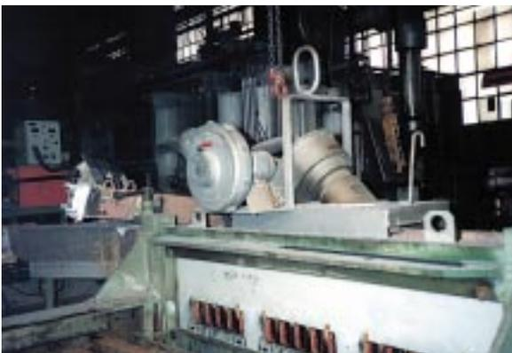
A Heater 40000 and ASO blower used to heat an aluminium extrusion prees. Hot air is also used to dry sand and burn out polystyrene cores in the foundry.
