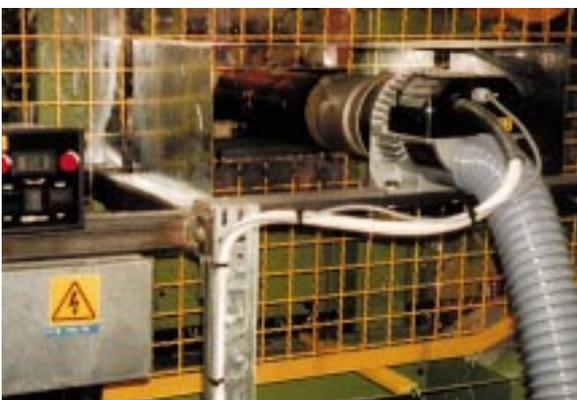
To prevent laminated glass material from sticking to the conveyor belt, it is heated on both sides by two Heaters 10 000 S with two tubular nozzles (1.2 m long). The KSR ensures the precision necessary for this heating process.
