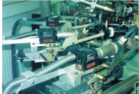
The coils of transformers and motors are often wound with self-bonding wire. The melting of the wire during winding is achieved by means of a finely concentrated stream of hot air.
