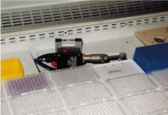
A Heater 700 hot air tool and Robust blower used to sterilise test needles.
