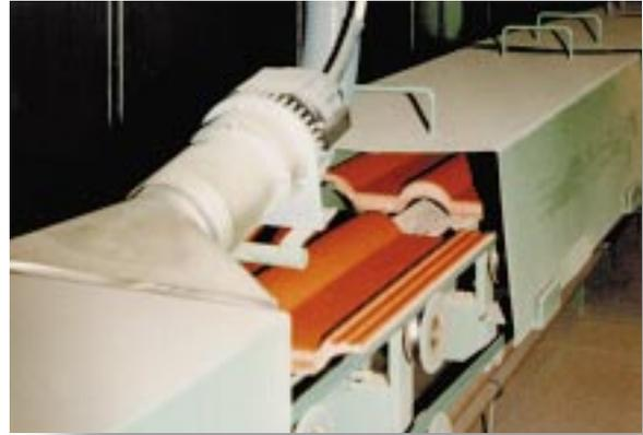
Six Heaters 10000 S and two ASO blowers in a drying tunnel. Coated roofing tiles are dried at high throughput speeds.
