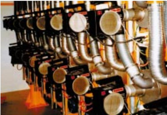
20 Hotwind S in a testing facility for ball bearings. The life of the bearings is tested at a variety of temperatures and rates of revolutions.
