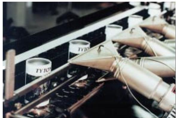
Six Heaters 5000 controlled by a KSR unit used to shrink PE sleeves on cans. High throughput speed and precise control ensure perfect shrink quality.
