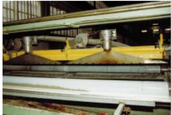
Two Heaters 40000 and two ASO blowers used to dry impregnated Eternit piping. Two wide slot nozzles (2000 mm long) ensure the air is evenly distributed.
