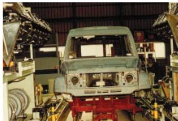
28 Heaters 10000 S used for curing adhesives. Instead of spot welding, the gutters are glued to the roof of this car. The watertight joint ensures that no rust can form and the channel can not be bent out of shape.
