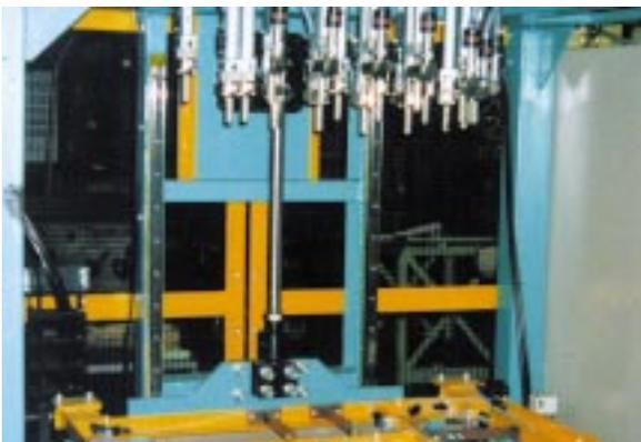
28 Labo 34 are used to heat up the rivets of plastic interior door pannelling. Subsequently the rivet, heads are formed using a cold punch.
