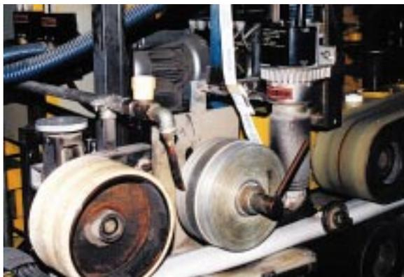
A Heater 5000 used to weld an endless PVC hose. The air is supplied by a Robust blower via an air flow off/on switch.
