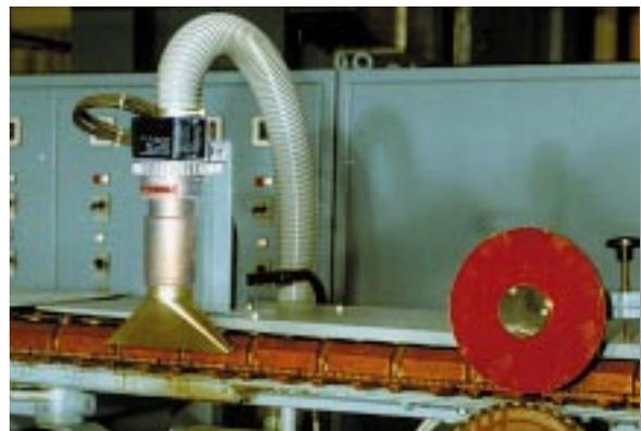
Drying the adhesive used to reinforce the edges of woven material. Even at high throughput speeds the material does not fray.
