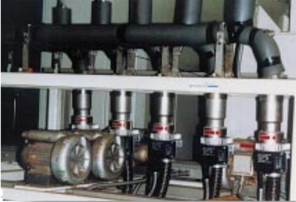
Five Heaters 5000 used to heat a tubular channel. Coated stranded steel wires are melted together as they are fed through the heated tubing.
