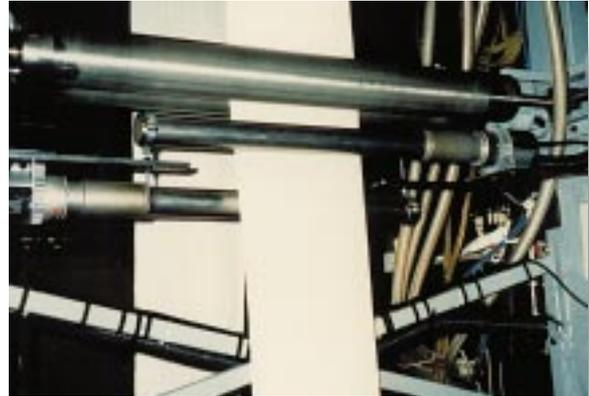
Two Heaters 5000 with space saving tubular nozzles (1.2 m long) for pre-warming paper prior to printing. The air is supplied by an ASO blower.
