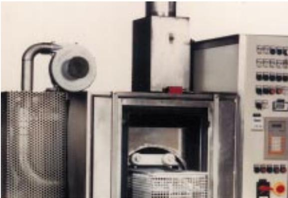
Automatic cleaning machines with environmentally friendly water based solutions use hot air to dry the washed articles. In small installations, the Heater 10000 S and the Silence blower are sufficient.
