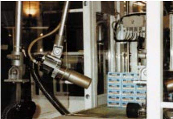
Two Heaters 5000 used to shrink packaging films on stacks of articles. At the end of the conveyor belt cold air is blown on to the heated areas by means of a Silence blower.
