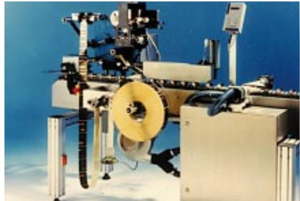
Two Heaters 3300 and a Silence blower used for shrinking covers on batteries, drying labels and sealing at high throughput speed.
