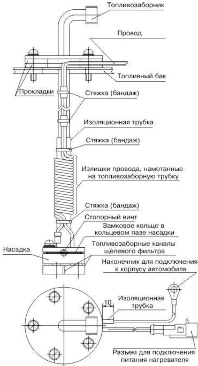
Fig. 1. Nozzle assembly on the fuel standpipe
