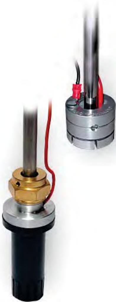
Heated fuel standpipe nozzles HTP-100 and HTP-200 are developed for installation on regular vehicular fuel standpipes to ensure diesel fuel intake from the tank under low temperature conditions when the intake of the frozen and condensed fuel is impossible by standard fuel standpipes. Diesel fuel pre-heating and accordingly its viscosity reduction and dewaxing before engine starting are conducted by the nozzle's electric heater operating on car battery (car system) power.
