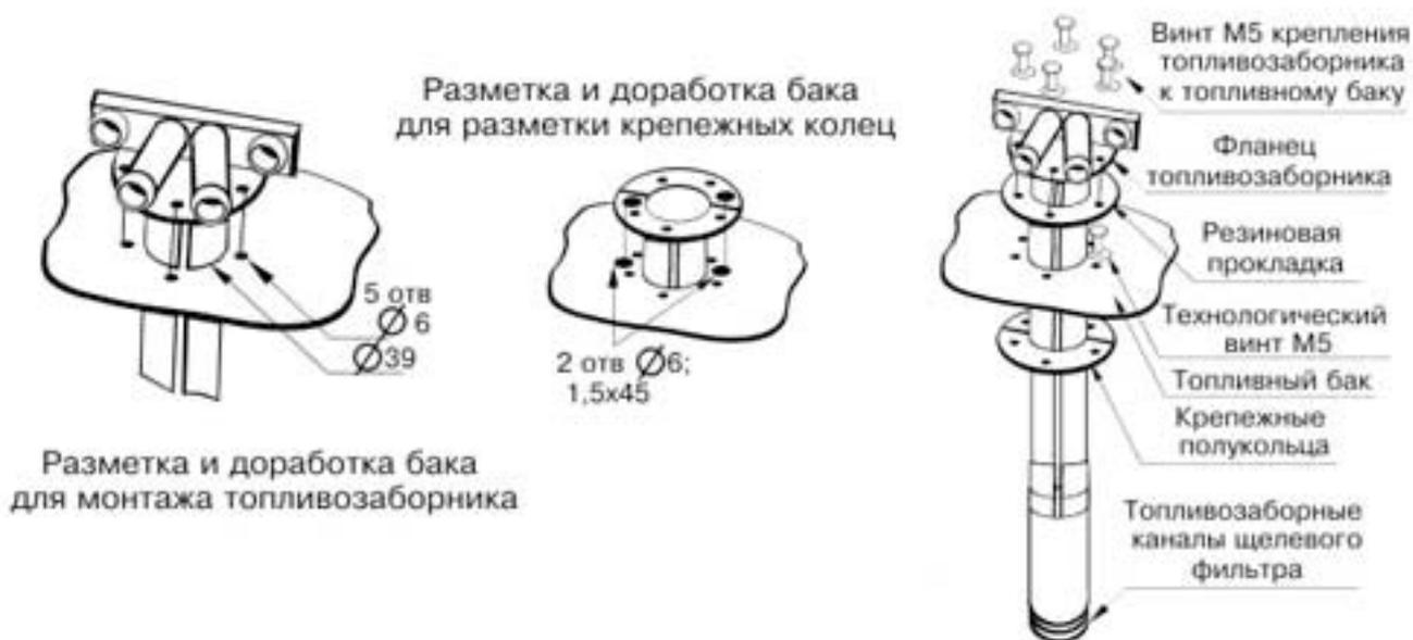
Fig. 1a. Nozzle assembly on the fuel standpipe TP-200
