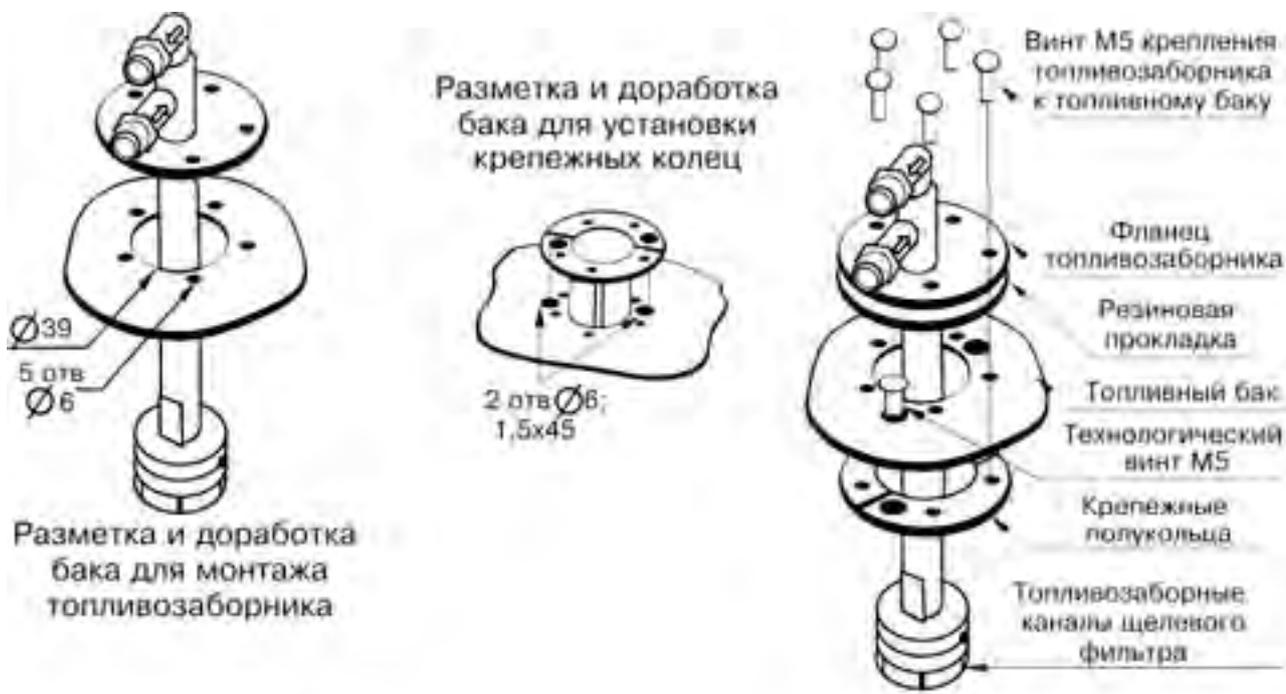
Fig. 1. Nozzle assembly on the fuel standpipe TP-100
