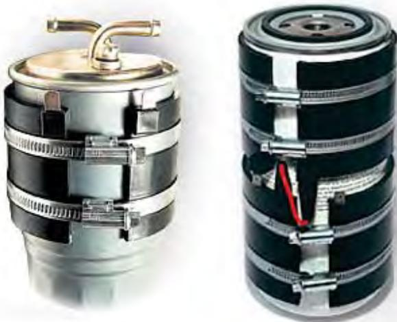
Electric strap (band) heaters ПБ-100 are implemented for the fine filter body pre-heating at the ambient temperature from  $-40$  to  $+5^{\circ}\text{C}$  to provide the required filter efficiency by fuel viscosity reduction and dissolution of the petroleum waxes formed therein under the temperature conditions below freezing.
