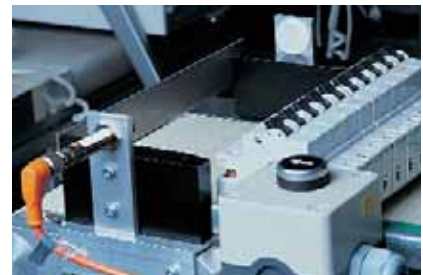
The reflector reflects the light beam: For a retro-reflective sensor transmitter and receiver are integrated into one housing.
