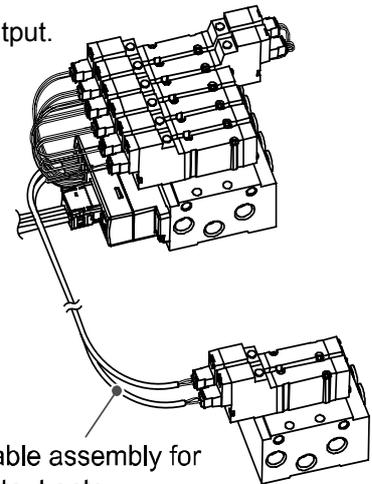
Cable assembly for output entry (EX510-V□□□)
