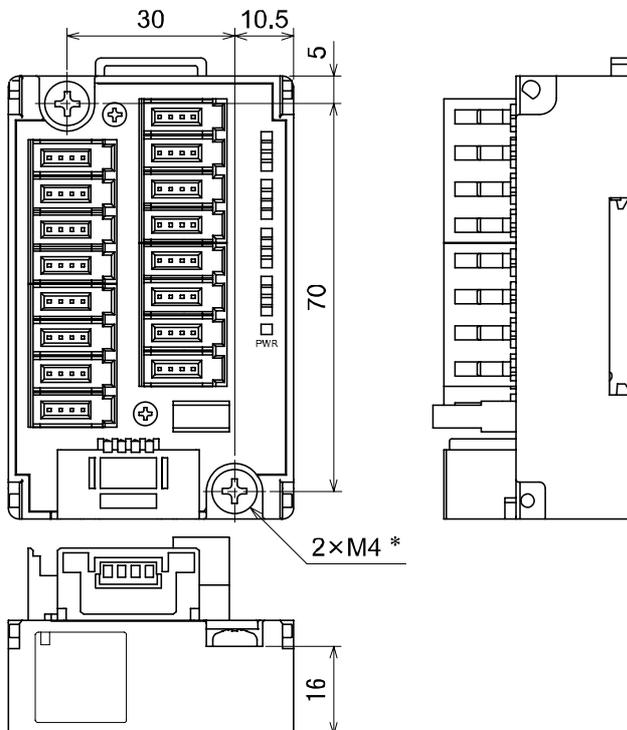
Cover removed (tolerance  $\pm 0.2$  mm)
