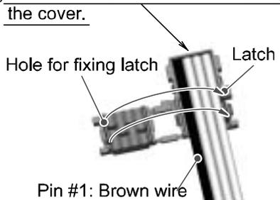
(3) Fold the cover so that the branch cable can be put between the cover.
