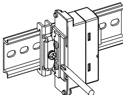
2, Tighten the screw by Phillips screw driver until DIN rail is secured. (Tightening torque: 0.6 Nm)
