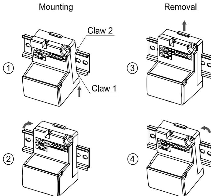
Put claw 1 of the body under DIN rail and push it upward. Push down Claw 2 to the opposite rail until the claw clicks securely on to rail. (Mounting procedure ① and ②)
