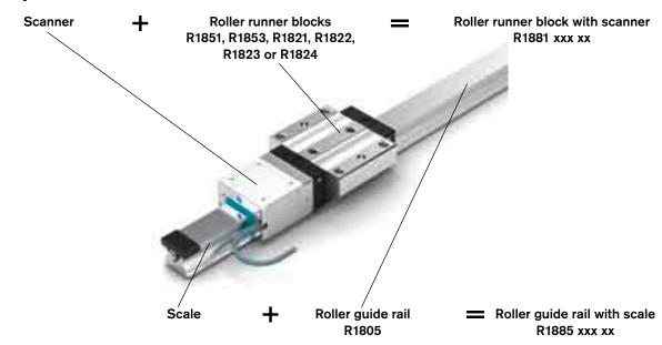
When Roller Rail Systems are ordered with integrated measuring system, the part number (PN) changes. A roller runner block with PN R1851, R1853, R1821, R1822, R1823 or R1824 is then given the PN R1881 to indicate that the scanner has been mounted. A similar procedure is followed when ordering the roller guide rail. The PN changes from R1805 to R1885 to indicate that the scale has been incorporated.
