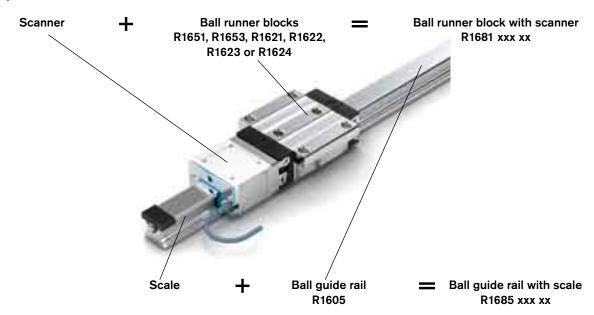
When Ball Rail Systems are ordered with integrated measuring system, the part number (PN) changes. A ball runner block with PN R1651, R1653, R1621, R1622, R1623 or R1624 is then given the PN R1681 to indicate that the scanner has been mounted. A similar procedure is followed when ordering the ball guide rail. The PN changes from R1605 to R1685 to indicate that the scale has been incorporated.
