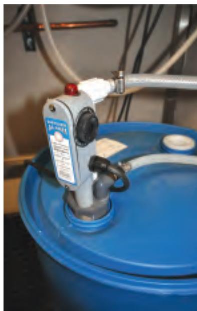
Pick-up tube with low level indicator
