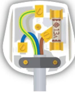
In the UK all modern appliances such as hairdryers, vacuum cleaners and microwaves use a square pin 13 amp plug. Plugs and their cables can suffer damage with use so it is a good idea to check them regularly.
