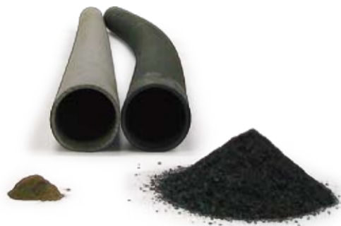
Fig. 4 Comparison of APMT Tube vs. Fe-35Ni-25Cr (after 2300 h at 1100°C (2010°F)). The FeNiCr tube is severely contaminated with oxide flakes.
