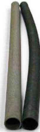
Fig. 2 KANTHAL APMT (left) and Fe-35Ni-25Cr (right) after the sagging test.
