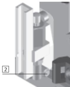
**2** The pressure piece guarantees freedom from backlash and precision at the end positions and in the effective linear stroke along the Z-axis.
