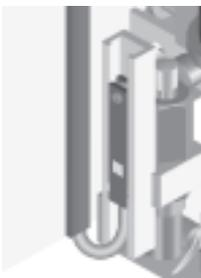
**1** Proximity sensor cables are installed via profile slots in the side and back plate.
