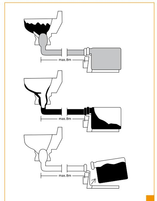
*Toilet and tank can be installed with a distance up to 8 meter.*
