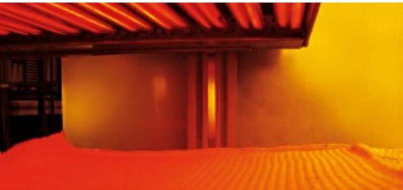
**Carbon twin emitters flow and cure powder coatings efficiently**
