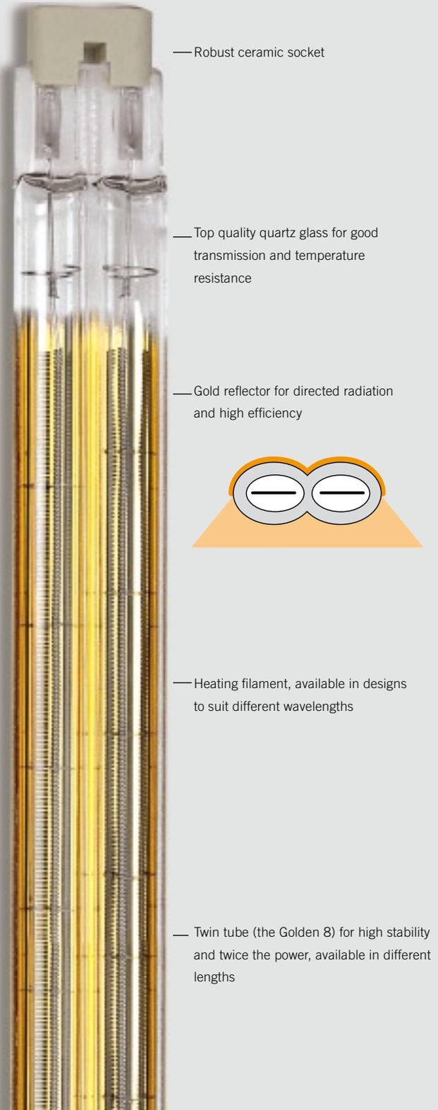
**Infrared emitters fixing innovative technical textiles**
