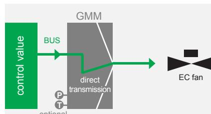
2.) no independent control is active – the control value that is preset via BUS is directly communicated to the fans. (slave signal)
