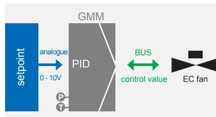
2.) automatic control to setpoint that is preset via analogue input
