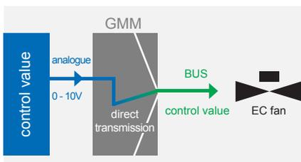
1.) no independent control is active – the control value that is preset via analogue input is directly communicated to the fans. (slave signal)
