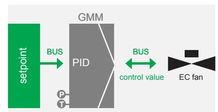
3.) automatic control to setpoint that is preset via BUS
