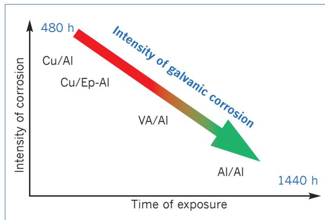
Test result (Salt spray test acc. to DIN EN ISO 9227 (DIN 50021)):
