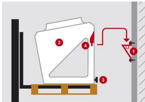
1. Attach mounting beam to wall
