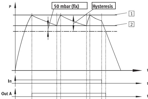
If the desired threshold [1] is reached for the vacuum, vacuum generation is automatically switched off. A non-return valve prevents the reduction of the vacuum. Nonetheless, leakages (due to e.g. rough workpiece surfaces) will
