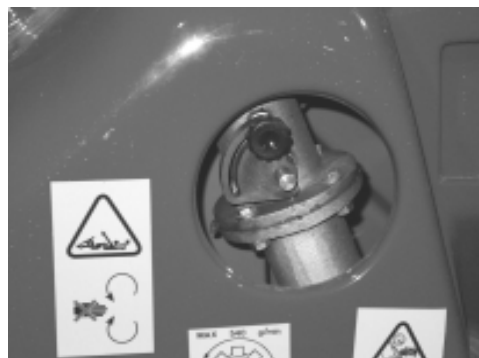
5. Speed is regulated by adjusting the by-pass
