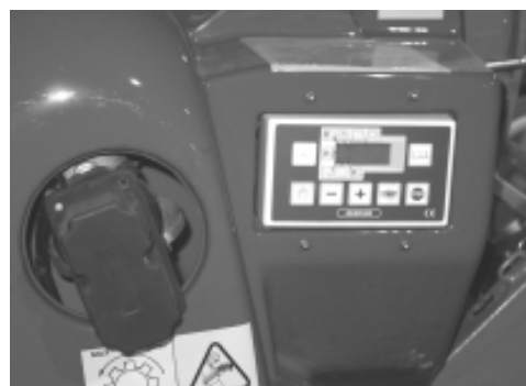
6. Electric motor regulates by-pass when using the optional GOLDEN RAIN computer
