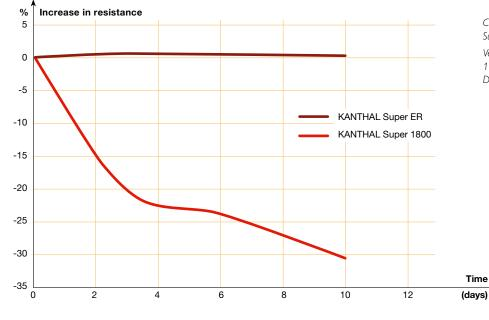
Corrosion properties KANTHAL Super ER vs. 1800 Velocity 1.7 m/s (3.8 mph) 100% H<sub>2</sub> at 1550°C (2820°F), Dp -40°C (-40°F)
