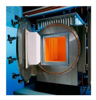
is often used. Operation in air or oxidizing atmospheres, however, is not possible due to the detrimental oxidation of molybdenum to  ${\rm MoO_3}$ .
