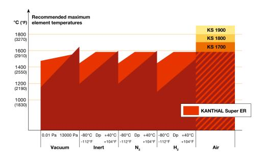
Recommended maximum element temperatures in different atmospheres
