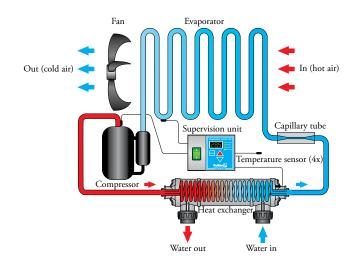
The actual pool temperature and the temperature of the refrigerant are shown in an LED display. The control unit has also a signal lamp for defrosting and is equipped with error codes.
