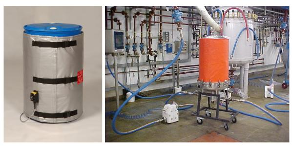
High Power Jacket for 205 litre drum, and chemically resistant jacket on process vessel
