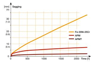
Figure 2 Comparative sagging test at 1100°C (2010°F).
