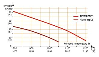
Figure 7 Power output SER-burner systems.
