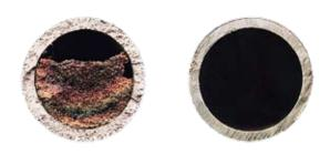
Figure 6 Comparison of carbon build-up in a strand annealing furnace, NiCr (left) and APM/APMT (right).
