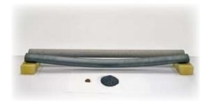
Figure 4 Comparison of APMT Tube vs. Fe-35Ni-25Cr (after 2300 h at 1100°C (2010°F)). The FeNiCr tube is severely contaminated with oxide flakes.
