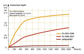
Figure 5 Carburization resistance.
