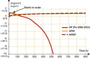
Figure 3b Sample weight gain – 1100°C (2010°F).
