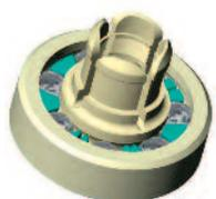
This device separates platelets from blood, which can later be used to speed the healing process of wounds or supply hemophiliacs with clotting factor. A bearing is used to provide rotary fluid exchange between the collection tray and the separator unit. The bearing operates at room temperature and rotates at 1,680 rpm without coming into direct contact with the blood. The existing bearing was too costly and experienced unacceptable field failures.
