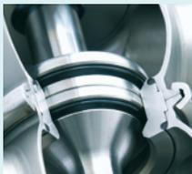
Trelleborg Sealing Solutions worked with the valve manufacturer from initial development of the product. By using FEA (Finite Element Analysis) and 3D modeling we identified the best geometry for an engineered seal to maximize sealing integrity. FKM V8605 was selected due to its chemical compatibility to production media as well as cleaning regimes and steam.
