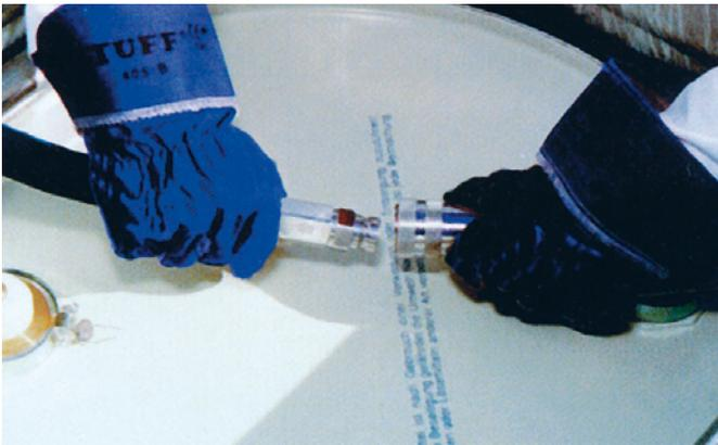
FDA and 3-A compliant EPDM E7502 was the ideal choice for secondary sealing, when an industry leading quick coupling manufacturer decided to develop a product for the chemical and beverage industry.
