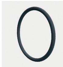
FEP O-Rings are an option when a seal with a high level of chemical compatibility is required. These consist of an elastomer inner ring encapsulated within a seamless Tetrafluoroethylene-Hexafluoropropylene (FEP) sheath. The FEP outer layer gives chemical resistance similar to PTFE, while a core
