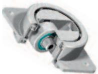
Comfortably moving patients in and out of the MRI machine is of utmost importance. The bearings used on the movable table must provide low friction and be non-metallic due to the strong magnetic field generated by the MRI process. The table bearings operate at room temperature and allow for 360 degrees of slow, smooth motion.
