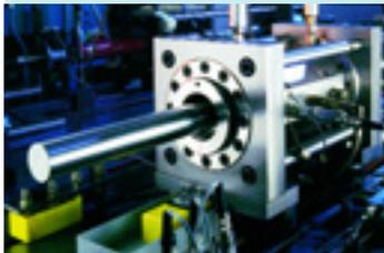
Figure 8: rod seal test rig
