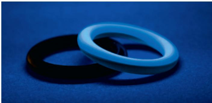
Uncoated and coated seal under UV-light
