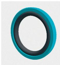
Turcon® Glyd Ring® and Turcon® Glyd Ring® T give excellent leakage control in piston and rod applications along with resistance to extrusion. These double acting O-Ring energized seals are primarily for dynamic applications where they give high wear resistance. Their low friction characteristics give
