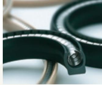
Wills Rings® are superior controlled-compression seals used for static applications. They are designed for extreme conditions, exceeding the capabilities of elastomer and polymer seals. Wills Rings® are made from high performance metallic materials such as stainless steel, copper, Inconel® or Monel® and coated with a softer metal or polymer.
