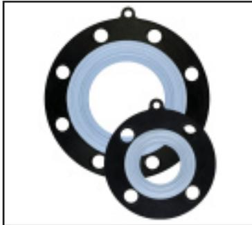
An Ansi Flex® (ANSI Flange 150#) gasket's contact surface is PTFE unitized to an EPDM rubber inner core. This totally bonded construction provides a PTFE gasket with the mechanical characteristics, including memory, of an elastomer gasket with exceptional steam resistance. An ANSI Flange 150# gasket is ideal for applications, such as PVC piping and glass lining pipings, where low seating stress is required.
