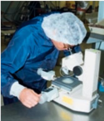
Trelleborg Sealing Solutions Hudson's primary focus is the manufacturing of precision products for the Life Science Market. It operates in a controlled environment equivalent to class 100,000 conditions, with ambient temperature, humidity, and particulate count monitored regularly. This facility follows strict "Good Manufacturing Practices"
