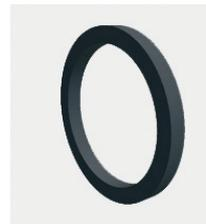
Trelleborg Sealing Solutions is the supplier of the original QUAD-RING®. This is a four lipped seal with a specially developed sealing profile. In contrast to the O-Ring, the QUAD-RING® avoids twisting in the groove, has improved friction characteristics and gives higher sealing efficiency in some applications.
