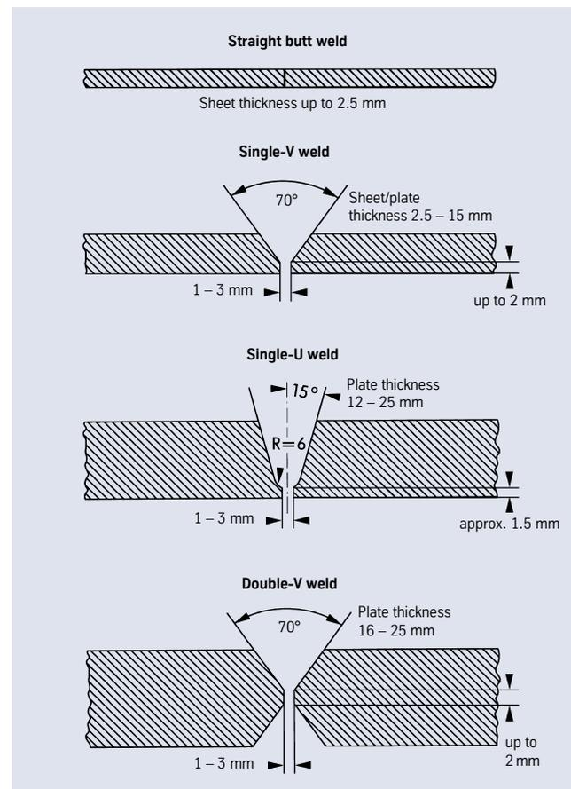
Fig. 5 – Edge preparation for welding of special stainless steels.
