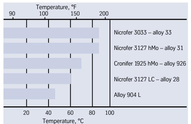
Fig. 3 – Critical pitting temperatures (CPT) of Nicrofer 3033 – alloy 33 and other special stainless steels, tested in 10 %  $FeCl_3 \cdot 6 H_2O$  solution for 24 hrs.
