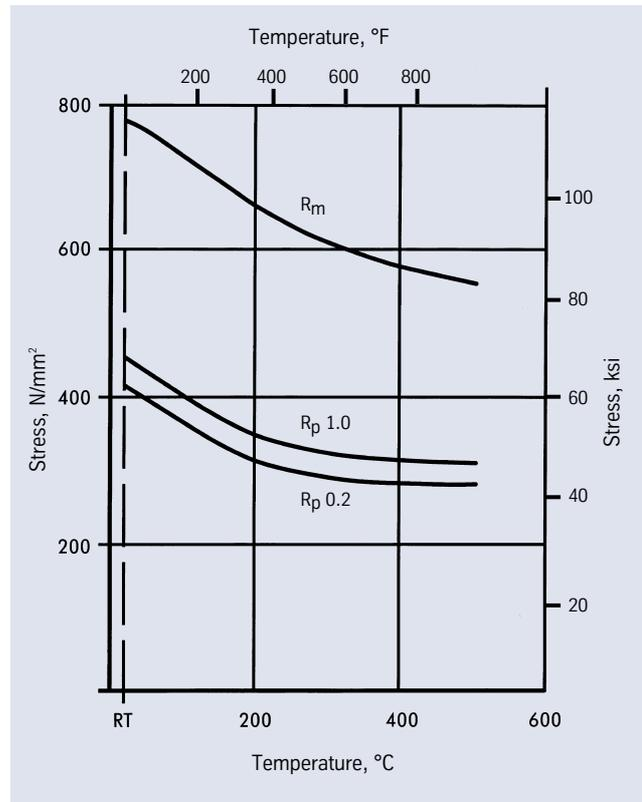
Fig. 1 – Typical mechanical properties of Nicrofer 3033 – alloy 33 sheets in the solution heat-treated condition.
