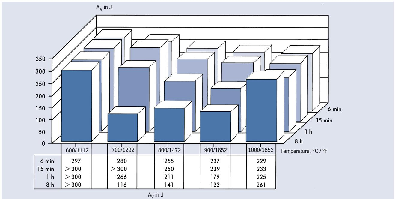
Fig. 2 – Time-temperature-impact strength diagram of Nicrofer 3033 – alloy 33, established on ISO-V-notch samples at ambient temperature; starting condition solution annealed,  $A_V > 300$  J. Typical values.
