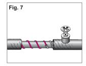
= Possibility of using 2 parallel cable lines instead of winding the cable around the pipe (see fig. 10).
