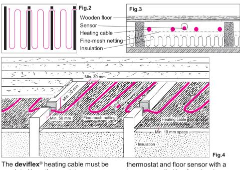
regulated by a thermostat. There must always be installed a thermostat and floor sensor with a temperature limiting function, i.e. **devireg**<sup>®</sup> 122 or **devireg**<sup>®</sup> 522.
