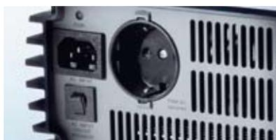
Front with input and mains input fuse
