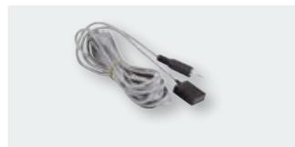
The IU0U chargers of series IU 152A to IU 802A can be equipped with a temperature sensor available as optional extra. The temperature sensor adjusts the charging voltage to the current battery temperature. This ensures a better charge at cold temperatures and prevents battery gassing at high temperatures.
