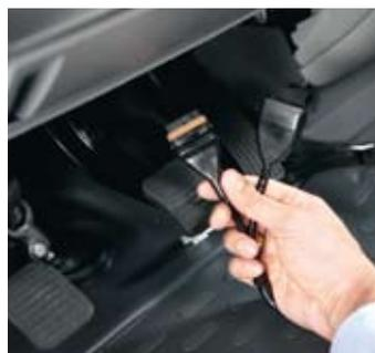
Connection to the accelerator via T-plug
