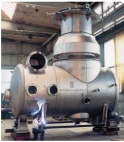
In petrochemicals, nickel-based alloys and high-temperature, creep-resistant stainless steels are needed for the production of plastics and synthetic fibers. The alloys' function is to extend the service-life of plant systems and individual components, prevent corrosion damage and ensure the purity of manufactured products.
