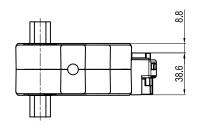
Min./max. operating pressure: 0,4 / 0,8 MPa Operating temperature: 5° + 45° C Opening angle: adjustable from 0° to 135° Electronic 24 Vdc sensor with M12 swivel connector that can be orientated at 0° or 90° Protection Class: IP 65 Pneumatic ports on both sides
