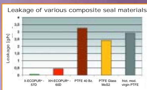
Fig. 4: Leakage of various composite seal materials
