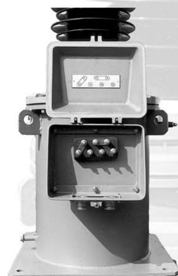
Secondary terminal box
