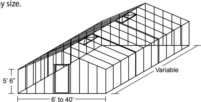
IGC glass greenhouses are also available with a curved eave and can be made to build on a knee-wall or glass to ground. Available in bronze, green or white. All IGC Glass Greenhouses are engineered to meet 70 mph wind and 10 pound live load per the UBC Building Code. For an additional expense, your structure can be designed to meet any building code requirements for live and/or wind load. Call IGC customer service for pricing on any custom requirements.
