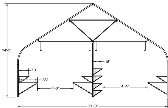
The Shelfmaster Teaching Package is NOT a load-rated structure, but features a sturdy, galvanized steel frame that easily snaps together. The structure can be secured with ground stakes on turf or weighted water tubes. The built-in benches make it a convenient all-in-one package. Call IGC customer service if you have questions or for pricing on any custom requirements.
