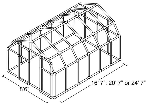
Features include UV protected PVC profiles and twin wall polycarbonate covering with a 10 year discoloration warranty. The Giant is covered with 4mm panels on the roof with 6mm on the side walls. This roof also tested to hold 1,100 pounds of snow but please note that these greenhouses are NOT load rated structures.
