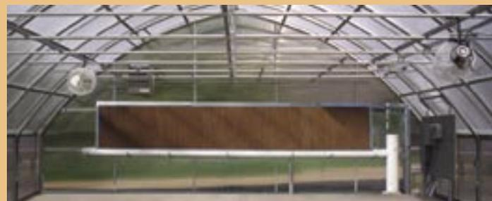
The Glacier-Cor PVC Cooling System is a complete evaporative cooling system with a 3' high wall and 4" pads. It works together with your greenhouse fans to lower temperatures 10-25 degrees. The sump is built-in and eliminates the need for a separate external sump tank, minimizing the amount of piping needed for the system.
