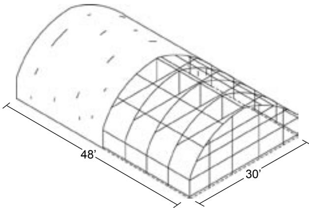
This greenhouse is engineered to meet 70 mph wind and 10 pound live load per the UBC Building Code. Higher load ratings and stamped engineered plans are available at extra cost. All galvanized steel frame insures maximum strength and life. Lexan twin-wall polycarbonate covering is UV resistant with a 10 year discoloration warranty.
