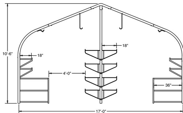
The Shelfmate Teaching Package is NOT a load-rated structure, but features a sturdy, galvanized steel frame that easily snaps together. The structure can be secured with ground stakes on turf or weighted water tubes. Horticultural classes can set up the Shelfmate greenhouse as needed and disassemble and store it when school's out. The built-in shelves make it a convenient all-in-one package. Call IGC customer service if you have questions or for pricing on any custom requirements.
