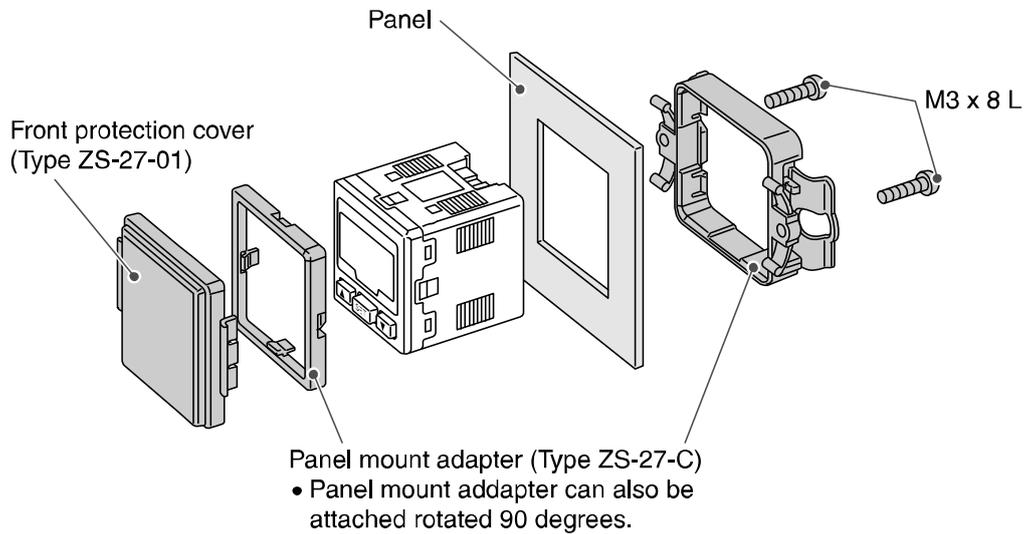
**Panel cut dimensions** Panel thickness: 0.5 to 6 mm
