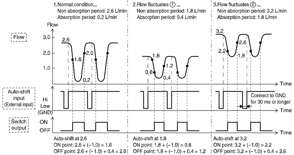
Table below shows the example of the flow display when auto-shift zero is selected. Here, takes normal condition as an example.
