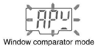
Set value is automatically calculated by pressing the button. The mode is changed to measurement mode. Once setting is performed, auto preset mode is turned off. It becomes possible to confirm the set value by pressing the button and perform fine adjustment of set value.
